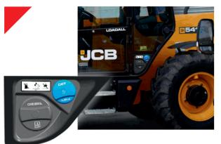
Locate & identify the diesel & AdBlue® fillers. AdBlue filler has a BLUE cap.
