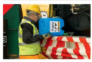
Fill the AdBlue® tank using only high quality AdBlue® conforming to ISO 22241.1 available from Scot-JCB.
