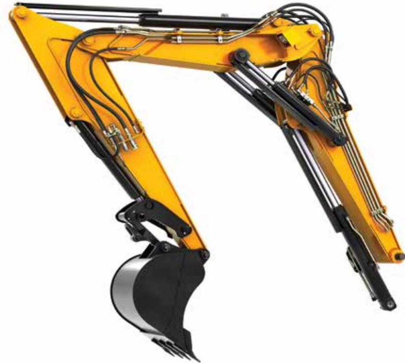
For ultimate lift capacity and stability, opt for our 86c with its optional triple articulated boom (TAB) giving you a greater working range with extended reach, closer digging and higher dumping capability.
