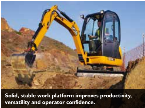
New dig-end geometry provides extra reach, load-over height, and dig depth.
