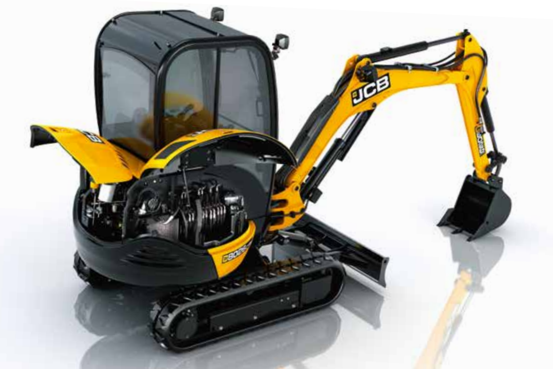
Pin end greasing makes lubricating the dig end quick and easy. While wide-opening service access panels are supported with gas struts for excellent access to routine checks.
