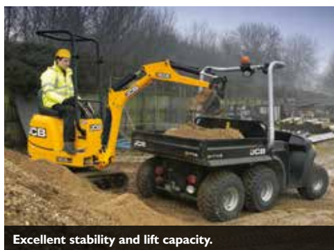
Compact size and minimal tailswing allows operation in confined areas.
