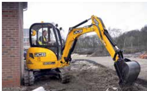
Slew and boom offset can be controlled simultaneously for faster machine positioning.
