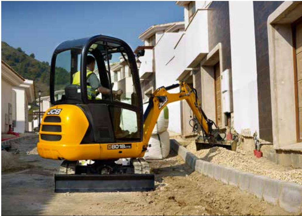
New dig-end geometry provides extra reach, load-over height, and dig depth.
