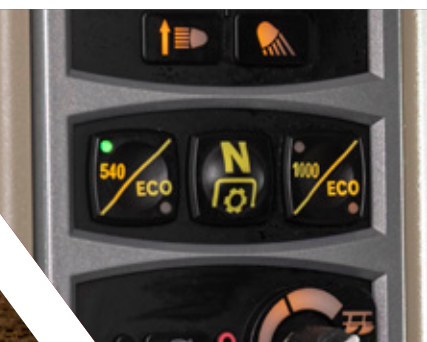
Electro-hydraulic PTO speed selection
