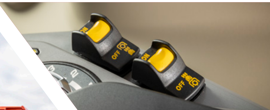
Electro-hydraulic PTO speed selection
