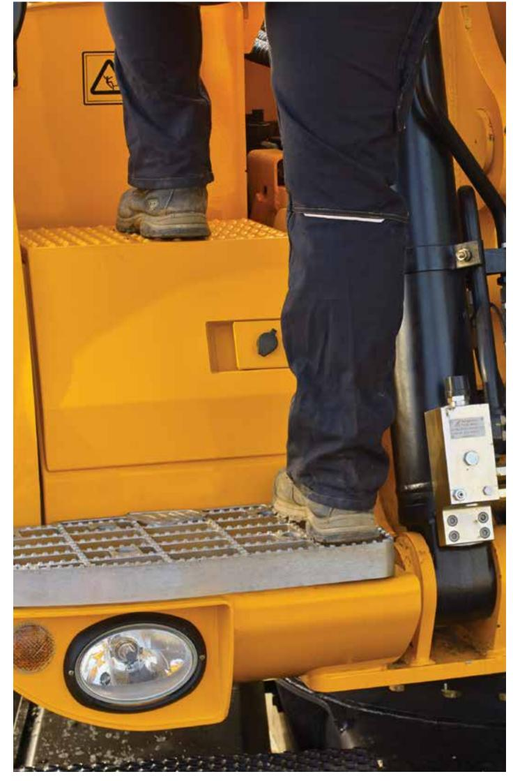
Standard safety features include: anti-slip surfaces, rear cameras, plus the JCB 2GO system.
